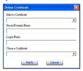
WPA uses 802.1x and Extensible Authentication Protocol (EAP) as the basis of its authentication mechanism. Thus your computer needs to install a certification for the RADIUS server first. Please consult with your network administrator for getting the certification and the appropriate parameters of the above screen.
